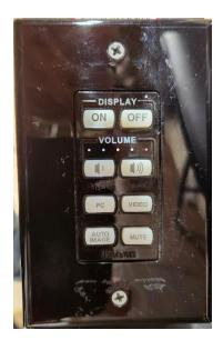
When finished using the equipment, please remember to turn off the projector by pressing the "OFF" button on the Extron controller.
