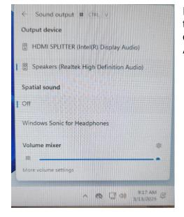
If another playback device is displayed, click on the speaker icon to select the correct device. Then click the arrow next to the name of the device and choose "Speakers (Realtek High Definition Audio).
